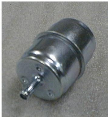
1. Loosen the hose clamps on either side of the filter.
