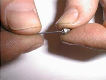
4. Re-install filters and orifices.
