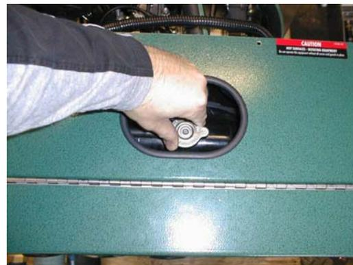
3. When adding coolant to the system, use a mixture of 50% antifreeze and 50% distilled water.
