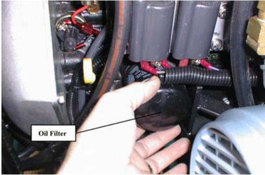
3. Apply oil to the new oil filter gasket. Install oil filter.
